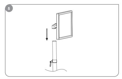
Lift the plate connecting part along with the monitor and put it on the locating ring.
