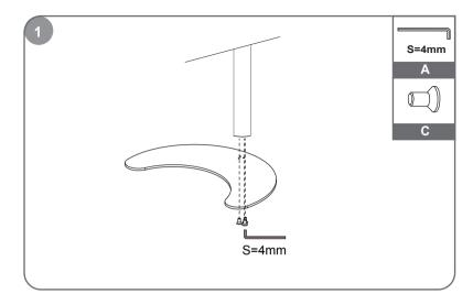
Use screws to connect the base with the steel pipe.
