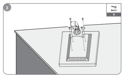
Flush surface installation: Install 4 screws through faceplate to monitor via mounting holes.
