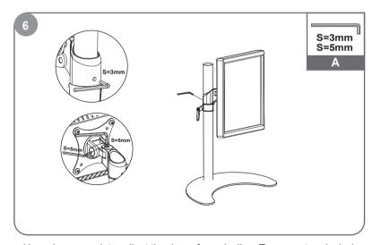
Use a hex wrench to adjust the damp for swiveling. Turn counter-clockwise to reduce damping and clockwise to increase damping.
