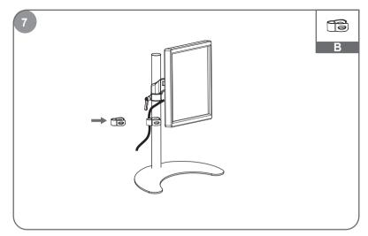
Use cable clamp to limit cables close to steel pipe.
